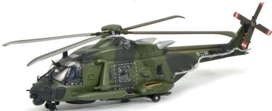
*The NH 90 (Nato Helicopter 90) was designed as a lightweight, all-weather and night-time multirole helicopter. Since the fuselage consists mainly of fibre composites, this helicopter has a far smaller radar cross section than other helicopters. As a multirole helicopter, the NH90's spectrum of missions ranges from transportation of material and personnel, especially special forces, through to the evacuation of casualties from the battlefield*
